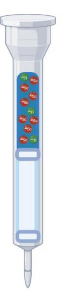
Production of  $^{45}$ Ti from  $^{45}$ Sc was achieved through irradiation of  $^{45}$ Sc target for 10 min at 10  $\mu$ A
