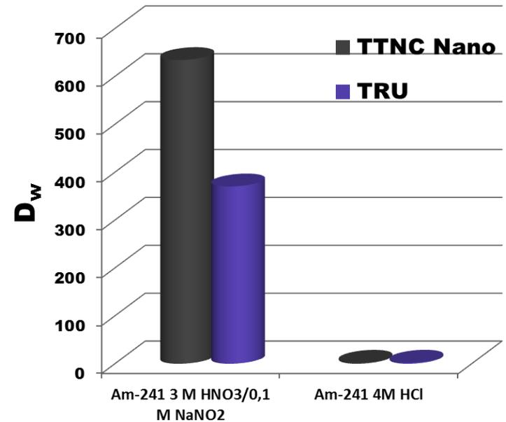
➤  $D_w$  significantly higher with carbon nanotubes compared to classical support
