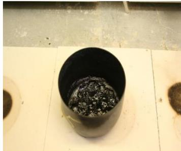
Wet ash residue with 15.8M HNO<sub>3</sub> and 30wt% H<sub>2</sub>O<sub>2</sub> on hot plate
