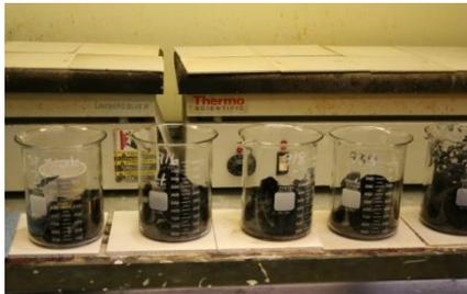
\* Routine analysis heating option to 550°C in 1 liter overnight without ceramic crucible
