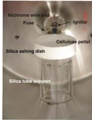
Sample loaded into disposable silica crucible
