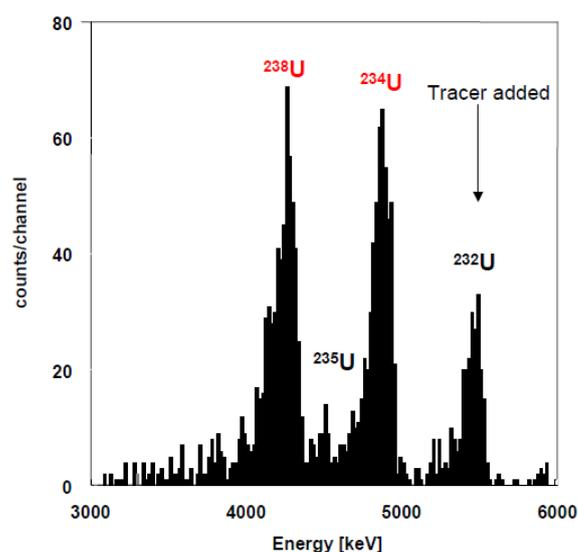
**Figure 3: Alpha spectrum of a mineral water sample ("Aproz Ancienne", Valais, Switzerland) obtained using a U-Nucfilm disc; Counting conditions: 900  $\text{mm}^2$  Si-detector at a distance of approx. 11 mm, acquisition time : 80'000 s. Added tracer activity is 200  $\text{mBq.L}^{-1}$ .**
