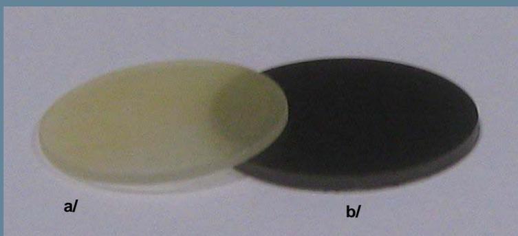
Figure 1 : a/ Ra NucFilm disc, b/ U Nucfilm disc
