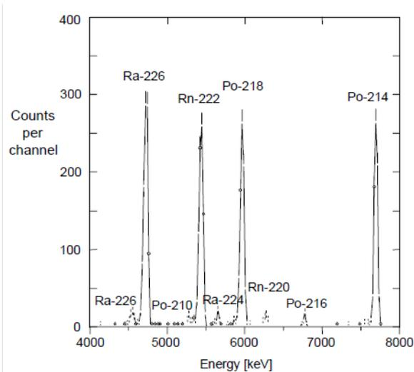
**Figure 2: Alpha spectrum of a radium adsorbing thin film exposed to a Portuguese mineral water.**
