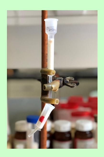
An isotope generator of Po-210 was prepared via selective sorption of Pb-210 onto the SR Resin column from 0.5 g of the REE concentrate dissolved in 30 mL of 3M HNO<sub>3</sub>.
