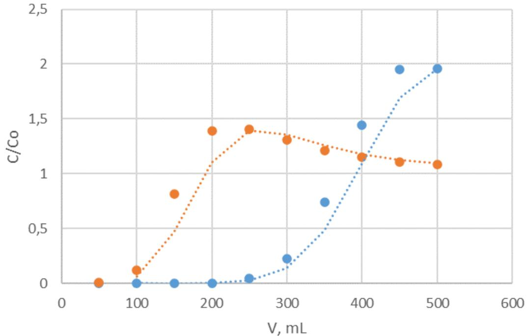
Fig. 29. Sorption curves of Cs and Rb on PR9 from seawater (pH 2).
