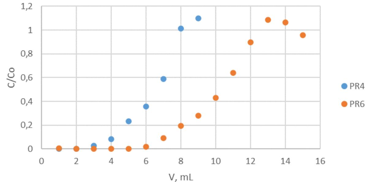
Fig. 14: Sorption curves of Cs on low-capacity prototypes in 3 M  $\text{HNO}_3$ . Initial concentration of Cs is 0,25 mg/mL.
