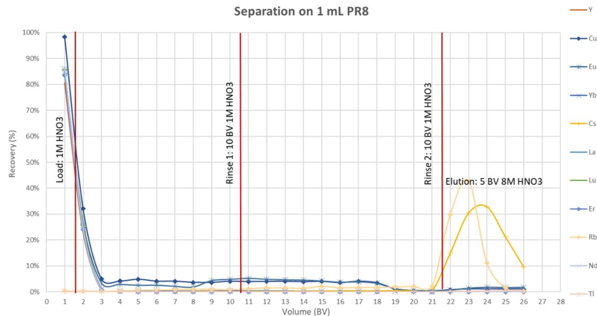
Fig 19: Separation of Rb and Cs on PR8 (loading in 1 M HNO<sub>3</sub> solution)
