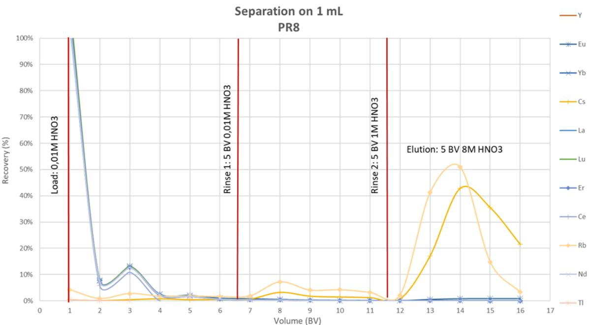
Fig. 18: Separation of Rb and Cs on PR8 (loading in 0,01 M HNO<sub>3</sub>)
