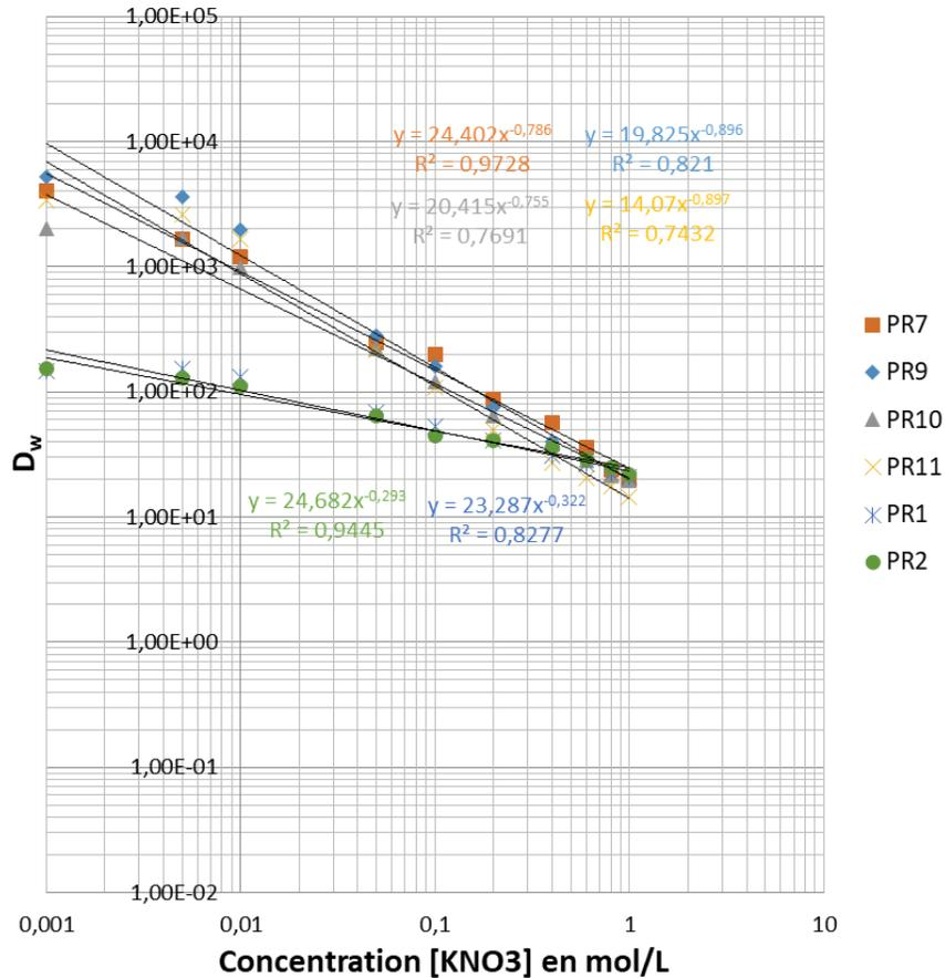
Fig. 7: KNO<sub>3</sub> dependency of Dw for Cs ion on high-capacity PR 1,2,7-11 in 1 M HNO<sub>3</sub>
