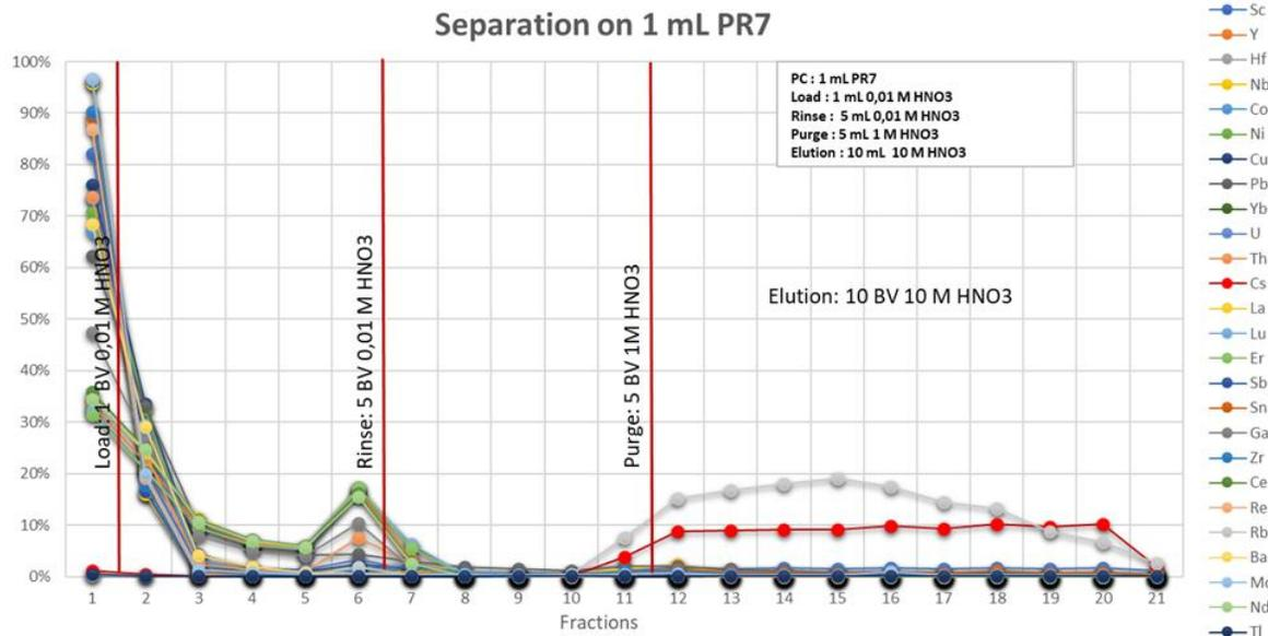
Fig. 20: Separation of Rb and Cs on PR7 (loading in 0,01 M HNO<sub>3</sub>)
