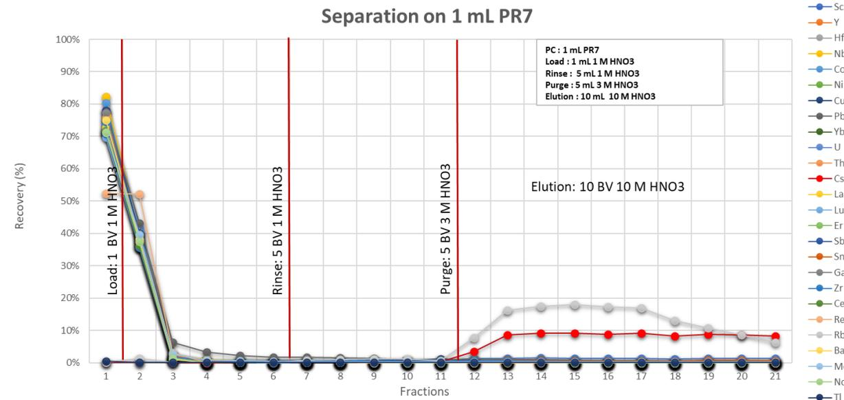
Fig. 21: Separation of Rb and Cs on PR7 (loading in 1 M HNO<sub>3</sub> solution)
