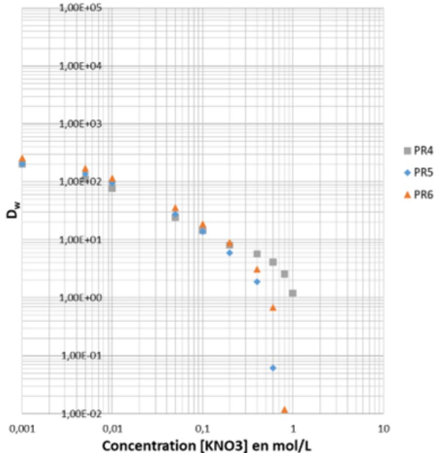
Fig. 9: KNO<sub>3</sub> dependency of efficiency of sorption on low-capacity PR 4-6 in 1 M HNO<sub>3</sub>
