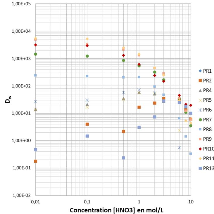
Fig. 2: Acid dependency of  $D_w$  for  $\text{Rb}^+$  on PR 1-13 in  $\text{HNO}_3$
