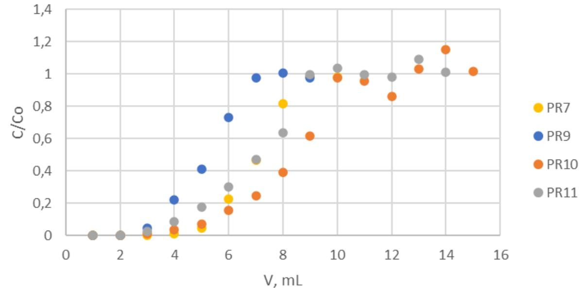
Fig. 16: Sorption curves of Cs on high-capacity prototypes in 1 M  $\text{HNO}_3$ . Initial concentration of Cs is 2,5 mg/mL.
