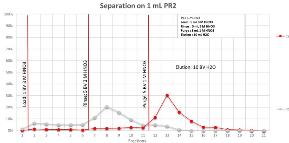
Fig. 24: Separation of **1000 µg** Rb and Cs on PR2
