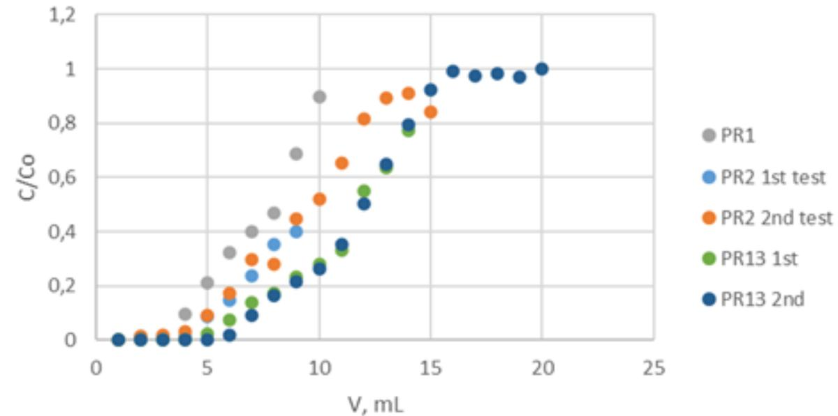
Fig. 11: Sorption curves of Rb on high-capacity prototypes in 3 M  $\text{HNO}_3$ . Initial concentration of Rb is 2,5 mg/mL.
