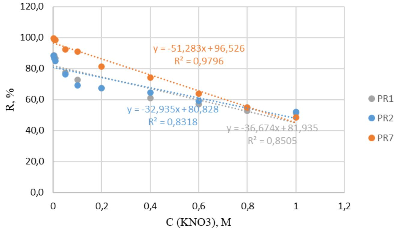
Fig. 8: KNO<sub>3</sub> dependency of efficiency of sorption on high-capacity PR 1,2,7 in 1 M HNO<sub>3</sub>
