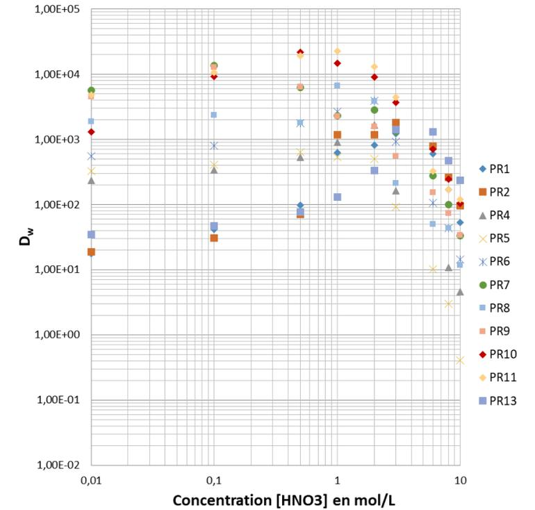
Fig. 3: Acid dependency of  $D_w$  for  $\text{Tl}^+$  on PR1-13 in  $\text{HNO}_3$
