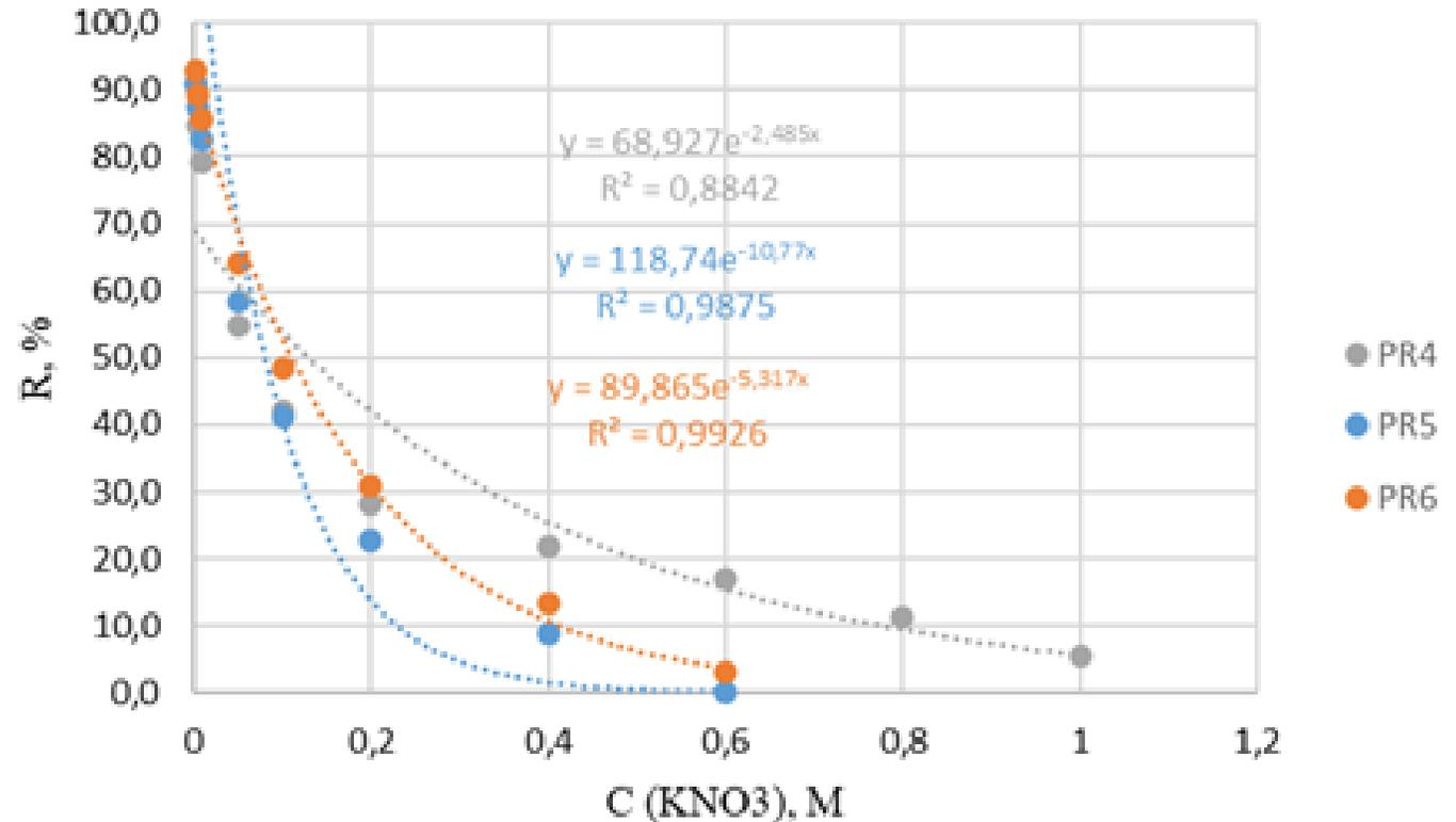
Fig. 10: KNO<sub>3</sub> dependency of efficiency of sorption on low-capacity PR 4-6 in 1 M HNO<sub>3</sub> in the presence of KNO<sub>3</sub>
