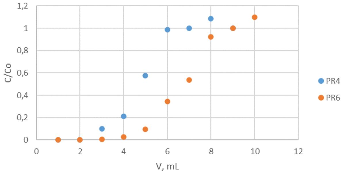
Fig. 13: Sorption curves of Rb on low-capacity prototypes in 3 M  $\text{HNO}_3$ . Initial concentration of Rb is 0,25 mg/mL.
