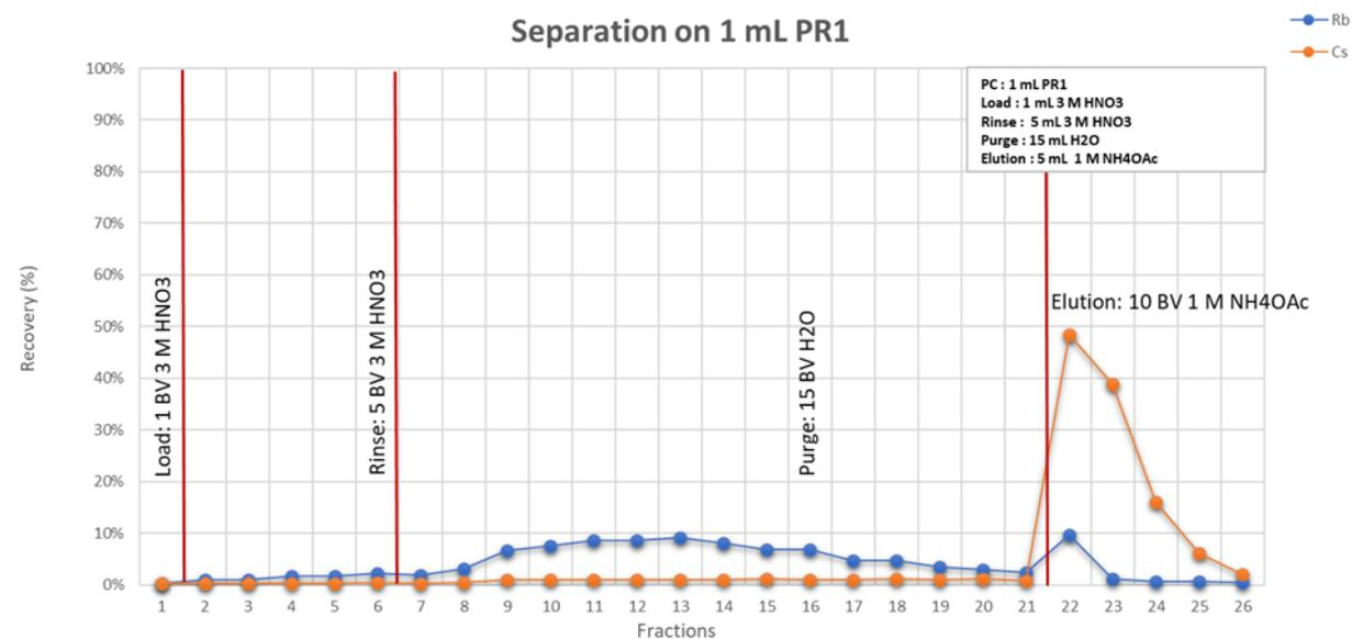
Fig. 26: Separation of 1  $\mu$ g Rb and Cs on PR1
