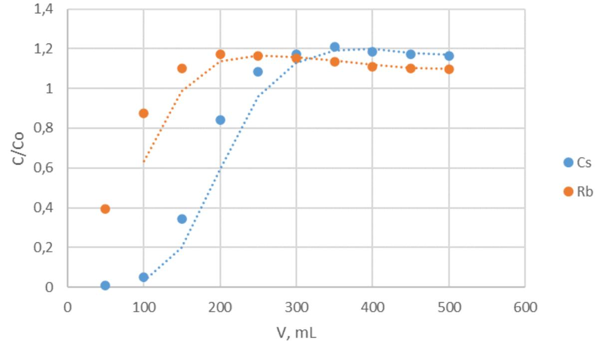
Fig. 28. Sorption curves of Cs and Rb on PR7 from seawater (pH 7,9).
