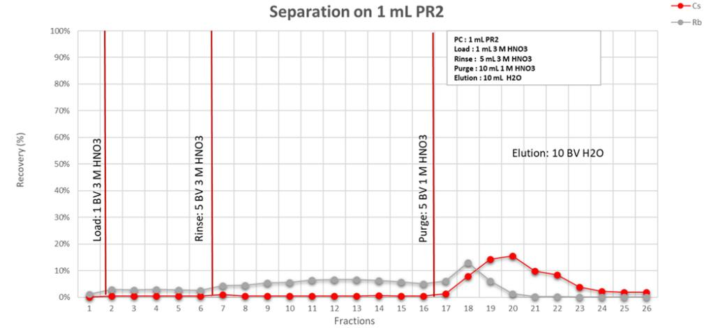
Fig. 23: Separation of **100 µg** Rb and Cs on PR2
