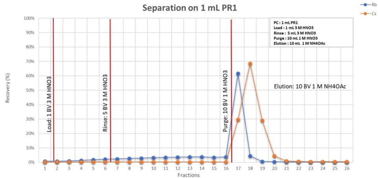
Fig. 25: Separation of 1  $\mu$ g Rb and Cs on PR1
