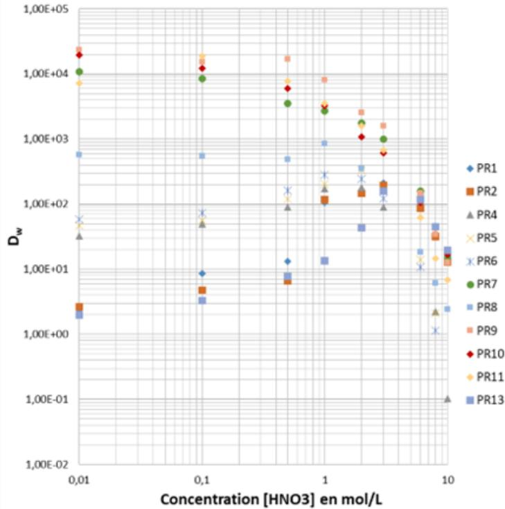
Fig. 1: Acid dependency of  $D_w$  for  $\text{Cs}^+$  on PR1-13 in  $\text{HNO}_3$
