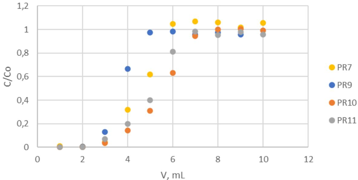
Fig. 15: Sorption curves of Rb on high-capacity prototypes in 1 M  $\text{HNO}_3$ . Initial concentration of Rb is 2,5 mg/mL.
