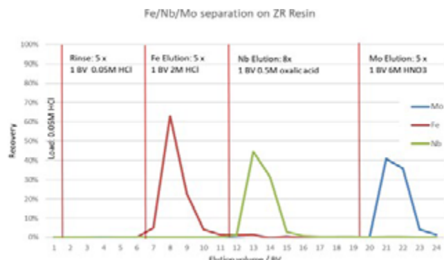
Fe, Nb and Mo separation on ZR Resin
